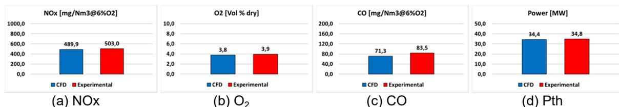
**Figure 11.** Experimental values (red bars) plotted against values from CFD analysis (blue bars).
