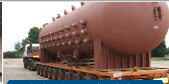
Boiler Drum being shipped from Gioia del Colle Factory
