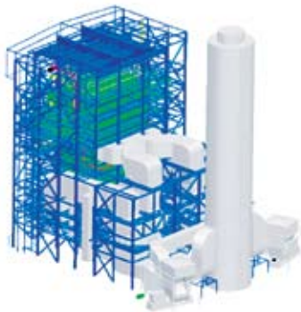
Abu Qir Power Plant (Egypt) 2x2,058 t/h gas/oil fired boilers
